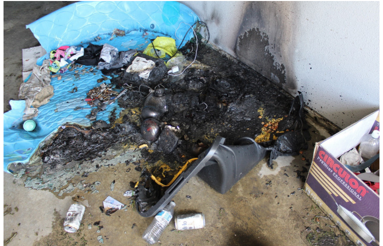
A heat lamp used in a garage to keep pets warm that started a fire.
